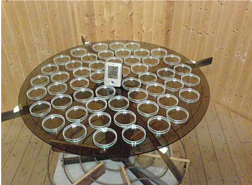
Fig. 3.1.1 Circular glass table with 52 dishes in the chamber at the Forschungsring Darmstadt.
