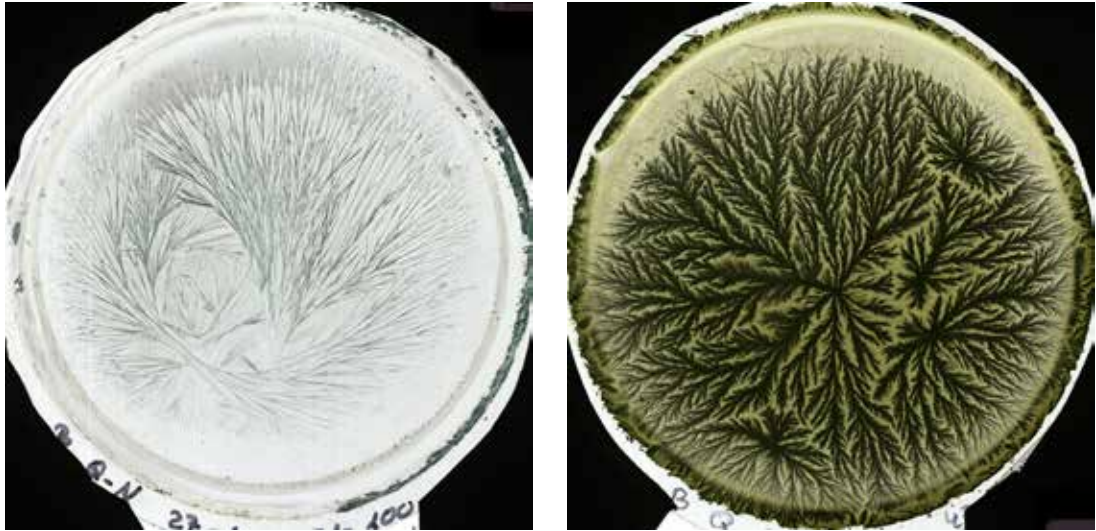
Fig. 2.16.1 Left: DCC with BSA displaying the split-growth crystal type. Right: DCC with BSA displaying the dendritic growth crystal type. Data from Busscher 2019 [17] Fig. 6, Fig. 7.
