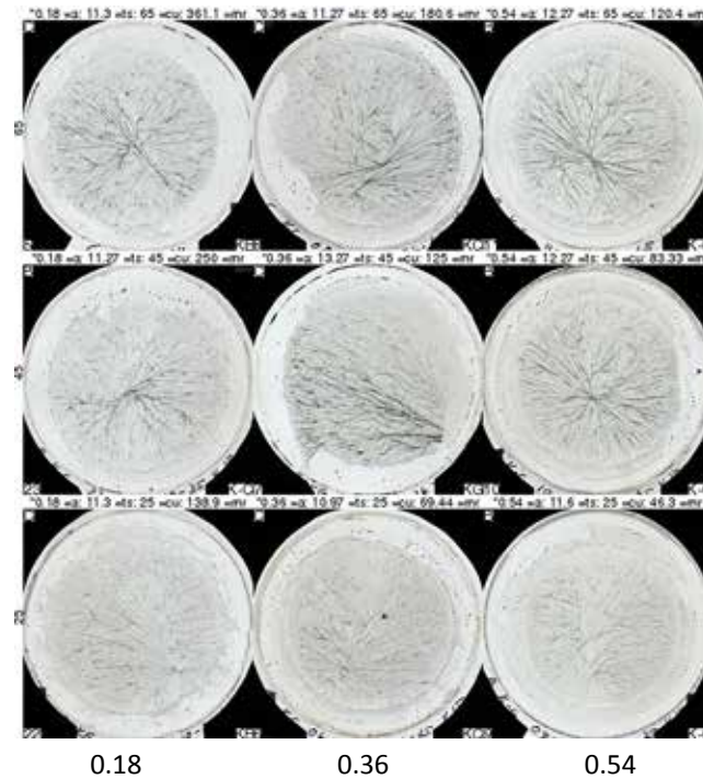
Fig. 2.6.9 PVP concentration matrix for K15 molecular weight. On the Y-axis is the DCC amount in mg per plate, on the X-axis the additive amount in mg per plate. Pictures University Kassel (D).
