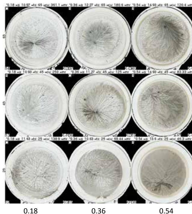
Fig. 2.6.6 PVP concentration matrix for K90 molecular weight. On the Y-axis is the DCC amount in mg per plate, on the X-axis the additive amount in mg per plate. Pictures University Kassel (D).
