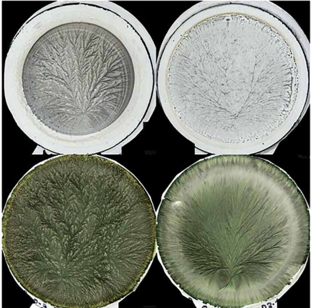
Fig. 2.6.2 Patterns from DCC crystallization with PVP K90 (top left, higher molecular weight), PVP K40 (top right, higher molecular weight), milk protein concentrate (bottom left, higher molecular weight) and whey protein concentrate (bottom right, higher molecular weight) as additives. From Kahl 2014 [9], Fig. 1).
