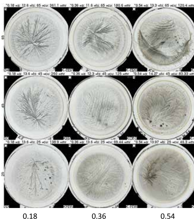
Fig. 2.6.7 PVP concentration matrix for K60 molecular weight. On the Y-axis is the DCC amount in mg per plate, on the X-axis the additive amount in mg per plate. Pictures University Kassel (D).
