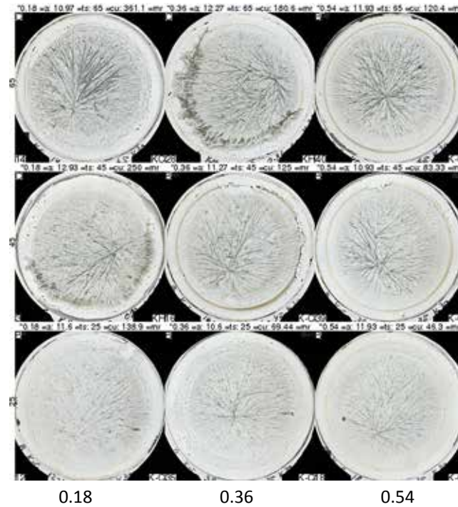
Fig. 2.6.8 PVP concentration matrix for K30 molecular weight. On the Y-axis is the DCC amount in mg per plate, on the X-axis the additive amount in mg per plate. Pictures University Kassel (D).
