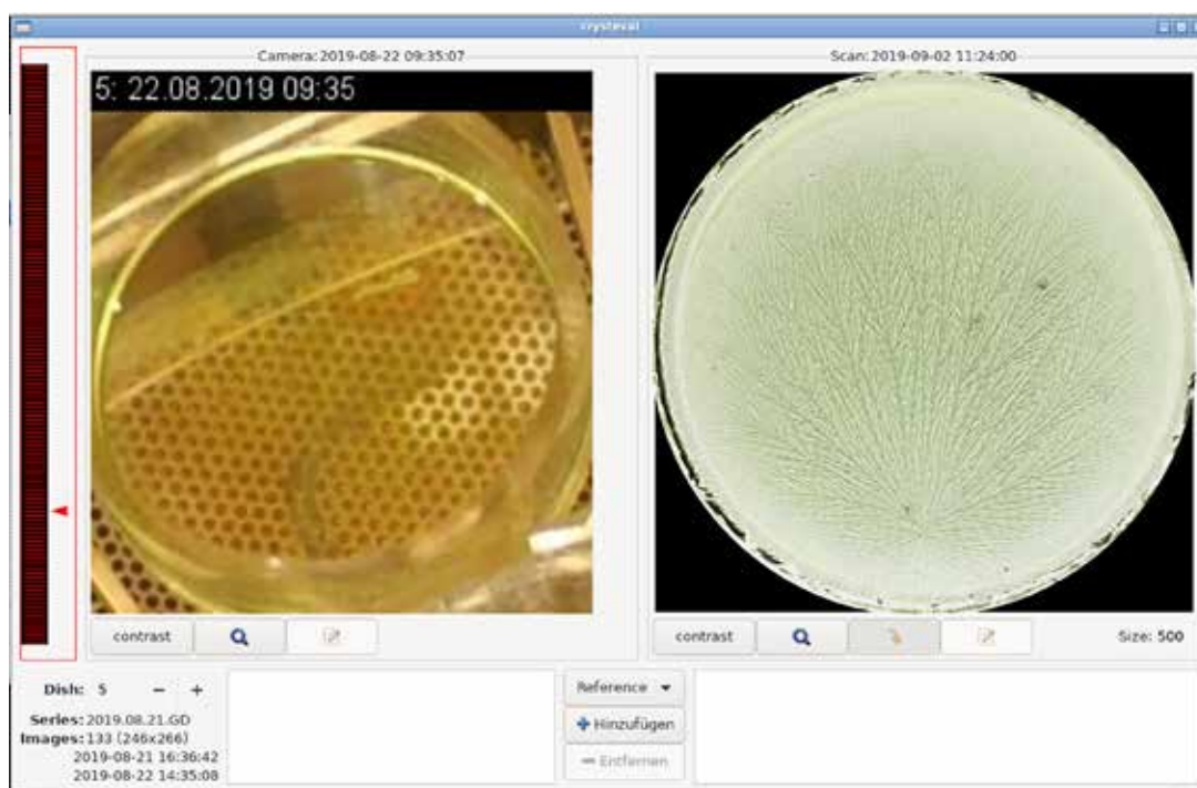
Fig. 3.3.2 Working level of CrystEval program for LabDoc series 2019.08.21.GD from chamber P for the dish at location no. 5 in the chamber (left), and the corresponding scanned picture (right).
