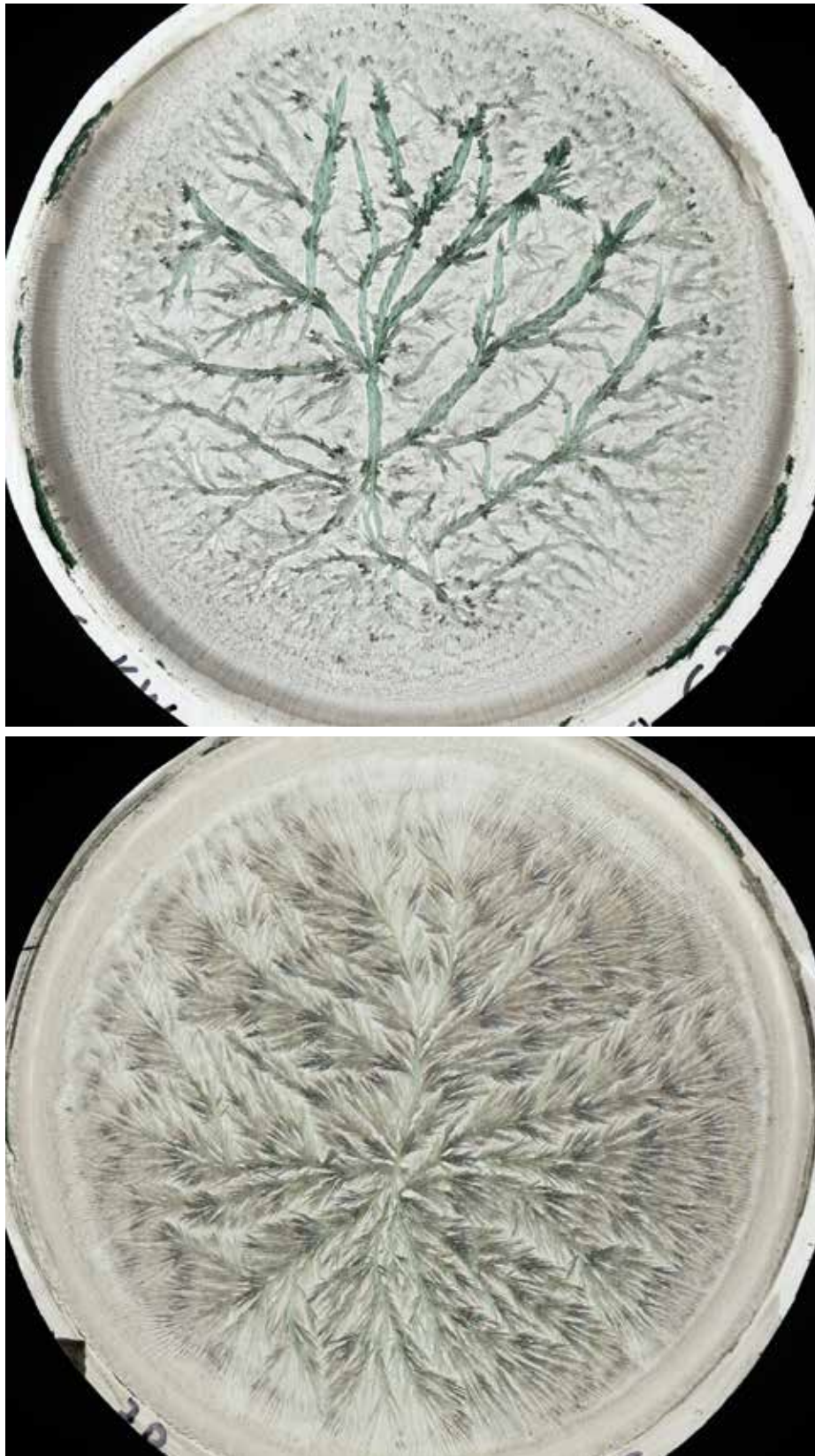
Fig. 2.9.1. DCC pictures with (upper picture) barley as additive ( DCC = 240 mg per plate, additive = 80 mg per plate) and (lower picture) wheat: DCC = 90 mg per plate, additive = 90 mg per plate. Pictures from University of Kassel (D) barley: LabDoc series C.2006.07.17.KW no. 11, wheat: DOK wheat, bio-dyn, LabDoc series C.2006.02.22.JP, no. 38.
