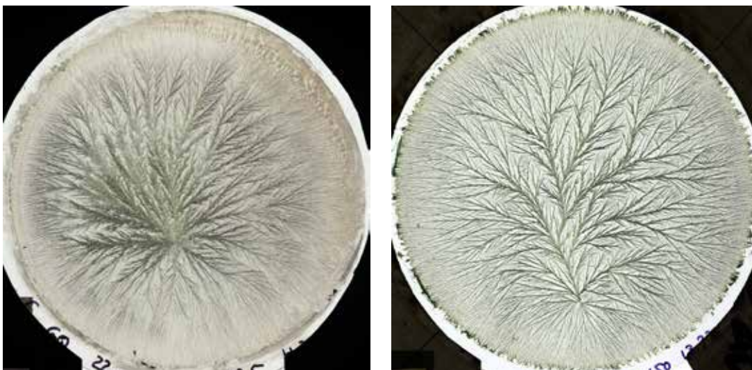
Fig. 2.15.1 Left: scanned DCC picture with apple juice as additive. Right: scanned DCC picture with cress extract as additive, showing the tree or plant-like structure from the crystallization start to the rim.
